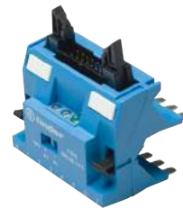
MasterADAPTER permits the easy connection of A1/A2 terminals to PLC outputs via a 14-Pole ribbon cable.
