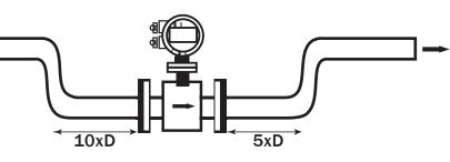
D= Diameter of Flow Meter in Inch
