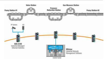
Under these circumstances, it is very difficult for operators to monitor the status of the switches at field sites and build the first layer of security for the network. Therefore, Moxa's recommendation was to upgrade the industrial networks at field sites with industrial managed Ethernet switches because they have enhanced security functions that fully comply with the company's security policy.
