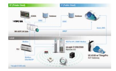
To deploy your I/O data to the cloud easily & effortlessly, you first need to retrieve the I/O data from the Local devices, then convert it to the appropriate protocol. Once all of the data has been prepared for transmission, the final step is to push the data up to your OT(Private Cloud) and/or IT(Public Cloud) platform.
