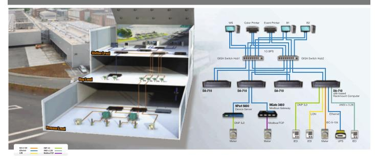
Substations typically have a lot of IED's meters & other devices sending data over multiple protocols including DNP3, IEC-101, IEC-103, & also converted to IEC-104 or IEC-61850. The computers & switches used in the substation now need to be IEC-61850 Compliant.
