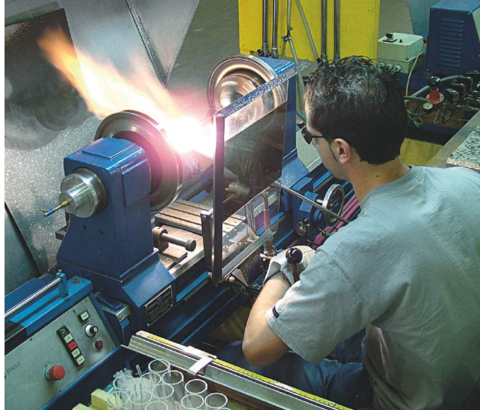
Shaping quartz glass lamp bodies
