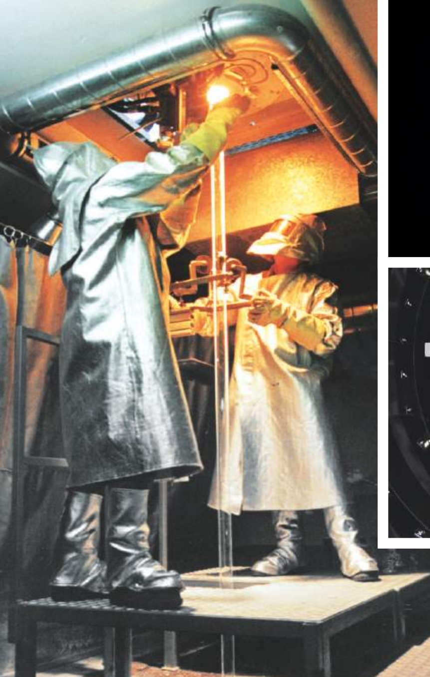
Furnace for quartz glass rods and tubing
