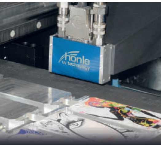
UV-LED curing of mobile phone casings
