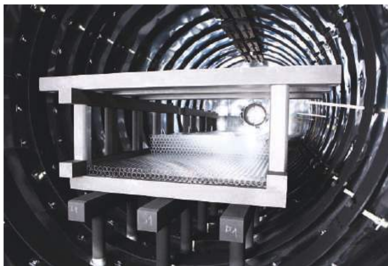
Vacuum annealing furnace for quality optimisation
