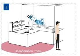
SafeSkin system detects when collision risk is eliminated, allowing seamless resumption of production program without manual intervention, enhancing human-robot collaboration efficiency.
