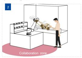
When an obstacle is detected by the SafeSkin, the CRAS collaborative robot is capable of activating its safety mechanism in just 0.01 seconds. Consequently, it promptly halts its operation within 0.1 seconds, effectively preventing collisions or minimizing the impact to enhance safety protection.
