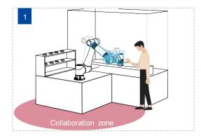
SafeSkin technology allows CRAS series robots to monitor human-machine collision risks in real-time. When the operator enters the collaboration zone, the robot can increase the maximum speed of collaboration up to 1 m/s\*, four times faster than traditional collision detection methods, while maintaining safety.
