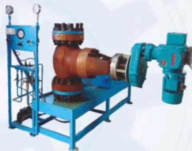
High Pressure Hydro Test Jig for Valve Testing
